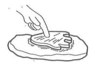
Step 3. Place model face down to make an impression into soil, glazing compound, or wet sand.
