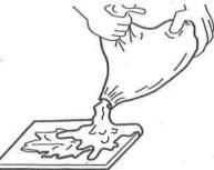
Step 4. Cut corner of bag with scissors and pour over mold.
